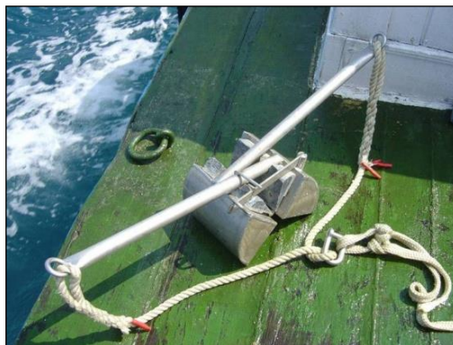
Figure 5.94 Van Veen grab sampler (left); Operation of a Van Veen grab sampler (right)
