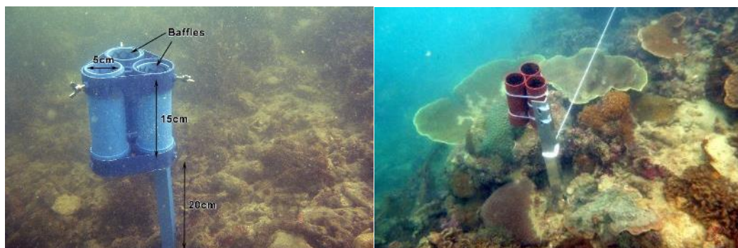
Figure 8.8 Examples of one set of sediment trap deployed along the reef crest
